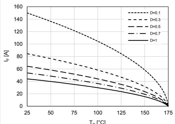
**Figure 3. Forward Characteristics**
