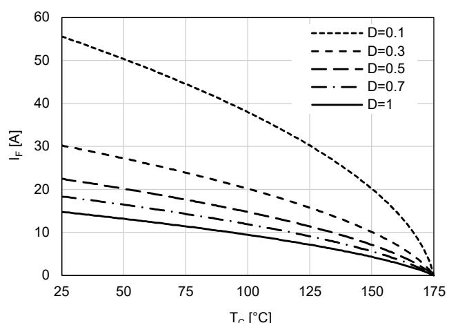
**Figure 3. Forward Characteristics**
