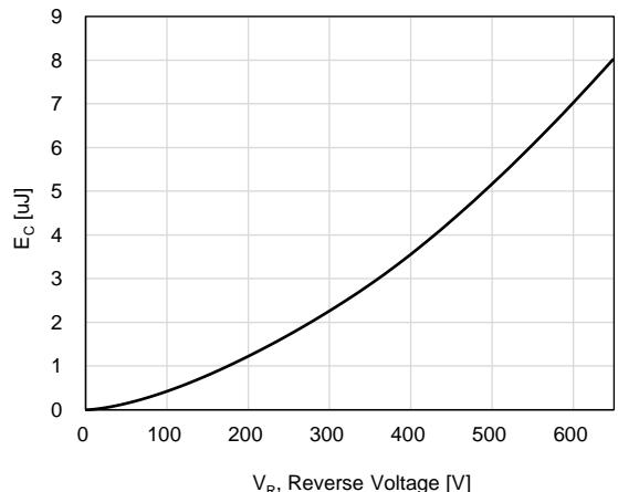
**Typical Performance Characteristics (Per Leg)****Figure 7. Capacitance Characteristic**
