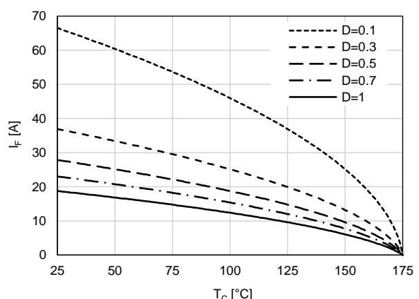
Figure 3. Forward Characteristics
