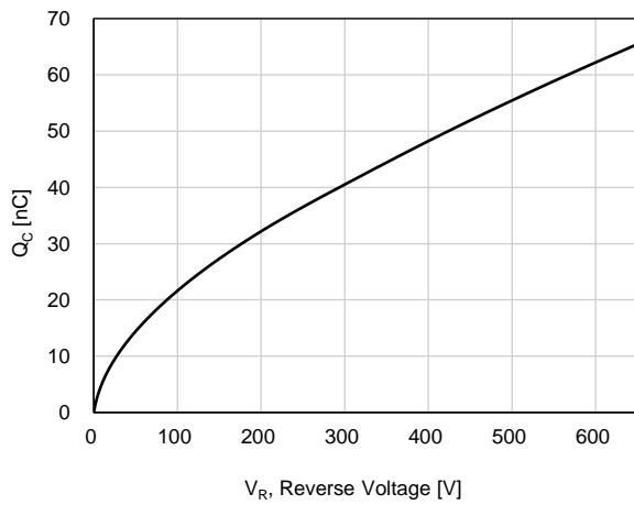
**Figure 6. Capacitance Stored Energy**
