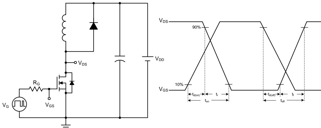
**Figure 14. Unclamped Inductive Switching Test Circuit and Waveforms**
